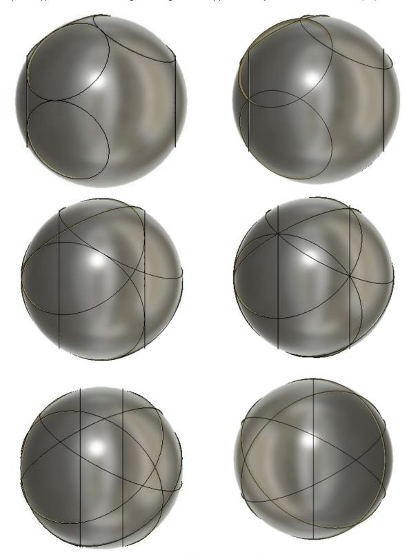
The savvy observer may recognize the source of this axis system's unique properties. Namely, this novel 8-armed jumbling axis system is neither novel nor jumbling; it is a face-centered platonic dodecahedral
