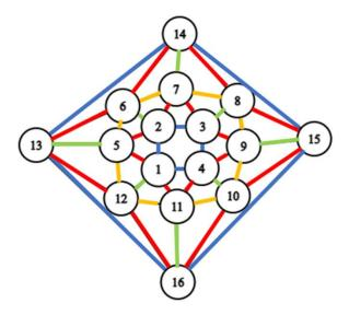
Three possible sets of dihedral edge length pairs based on the above subgroups are given below, along with a polyhedral mapping and cut depth spheres at 40 (shallow), 65 (medium), and 90 degrees (deep):
