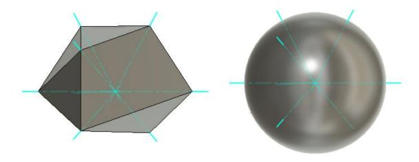
The piece-type critical revolve angles in degrees are approximately 31.7, 37.4, 58.3, 63.4, (75), and 90.
