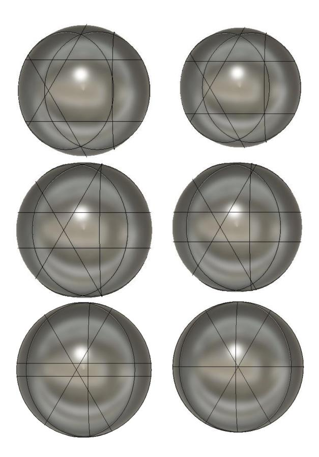
A puzzle with cut depths ~53 or ~76 degrees could make for an interesting puzzle. Both depths suffer from a disparity in piece size as well as multiple very small piece-types. This makes manufacture (especially at a reasonable size) difficult. Below is a 53-degree embodiment.
